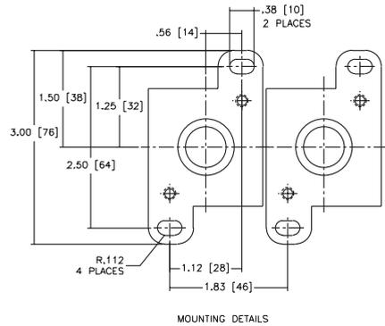
**Group-Mounted Construction - Dual Solenoid**
