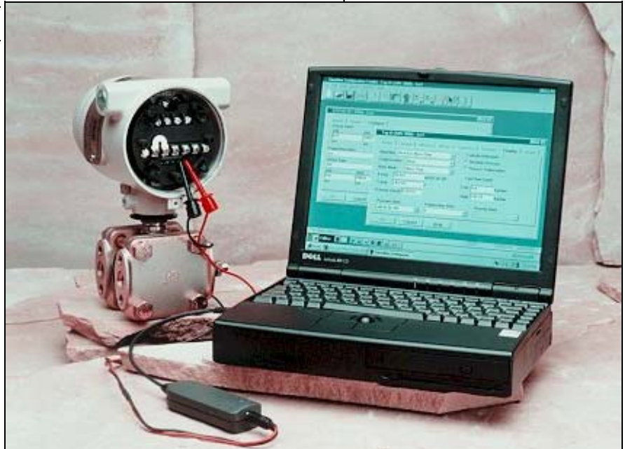
Figure 1 —SMV 3000 Smart Multivariable Flow Transmitter with SCT 3000 Smart Configuration Toolkit. The SMV 3000 measures differential pressure, static pressure and process temperature, and dynamically calculates mass or volumetric flow rate based on these measurements.
