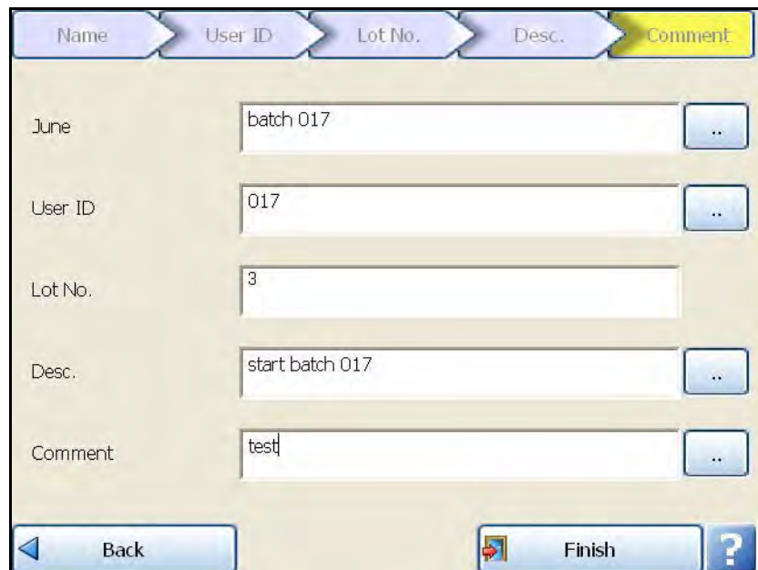
Figure 4.6 Batch Setup screens using Single Screen Batch
