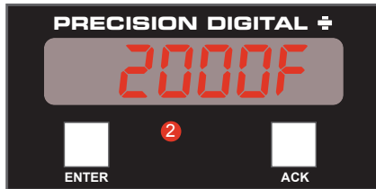
LED illuminated indicating that Alarm #2 is in alarm condition.
