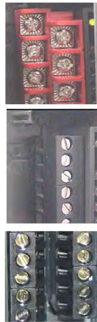
Terminal styles (top) Barrier (middle) Euro (bottom) 36-terminal Euro
