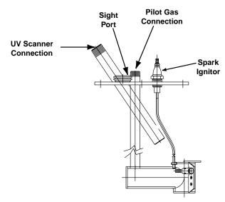
Refine pilot setting for a hard blue flame (and/ or strongest micro-amp signal) by adjusting gas flow through pilot regulator.
