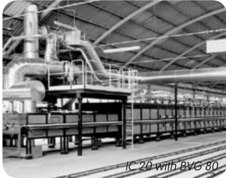
Roller hearth kiln in the ceramics industry
