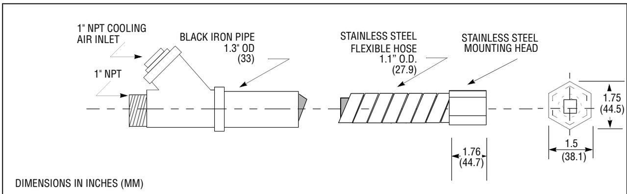
**FIGURE 3. INNER CARRIER ASSEMBLY**
