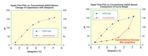
ture are about 600 times larger than that of conventional sensors. The larger sensitivity of HTF<sup>TM</sup> sensors makes Xentaur HTF<sup>TM</sup> more stable and almost completely immune to other influences, such as temperature, electrical noise and even long term drift. It puts Xentaur HTF<sup>TM</sup> sensors in a league by themselves.
